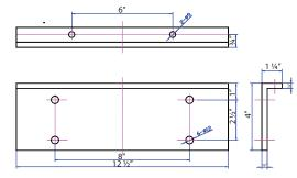
Steel bracket which is bolted to the upright steel frame
