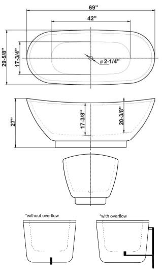
\*rough in center line 1" inch off outside of tub
