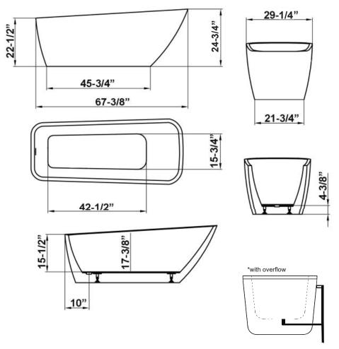
\*rough in center line 1" inch off outside of tub
