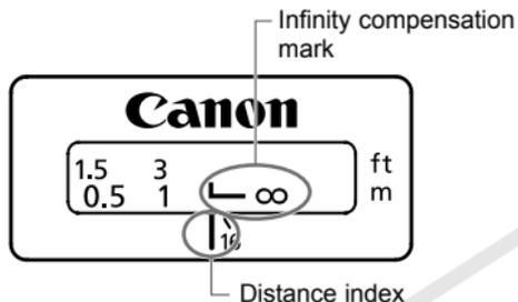
To compensate for shifting of the infinity focus point that results from changes in temperature. The infinity position at normal temperature is the point at which the vertical line of the distance scale L mark is aligned with the distance index.
