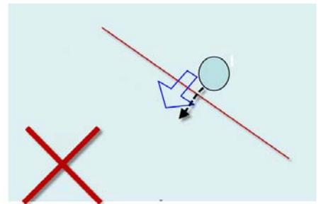
6. In order to maximize the accuracy and precision of this IVS function, please prevent targets from crossing the virtual detection line from the opposite directions at the same time. If there are two targets crossing the line simultaneously from the same direction without keeping safety distances, one count will only be recorded instead of two counts.
