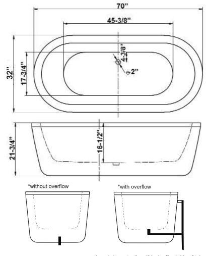
\*rough in center line 1" inch off outside of tub
