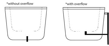
\*rough in center line 1" inch off outside of tub
