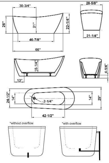
\*rough in center line 1" inch off outside of tub
