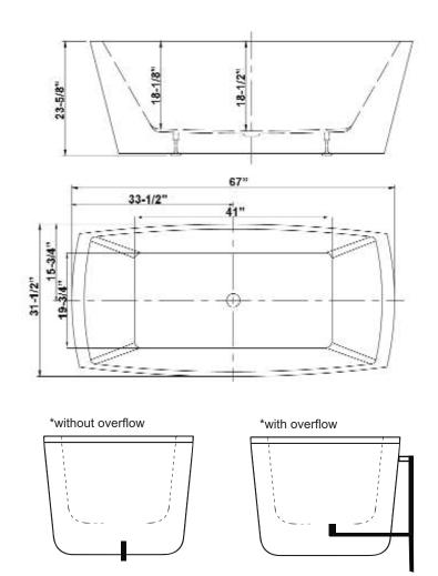
\*rough in center line 1" inch off outside of tub
