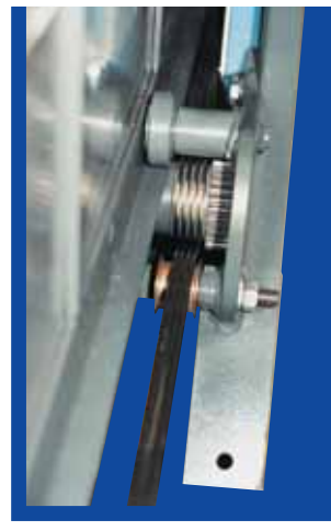
Overhead Cable Gear
