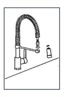
5. After intalling the faucet, remove spray assembly and open the hot and cold water supplies. Check for leaks. Turn on the faucet handle for one minute to flush debris from the faucet. Close the handles and re-assemble the spray.
