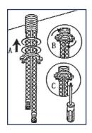
3. Re-assemble the mounting hardware onto the shank, use the philips screw driver for the final tightening after the spout is aligned.
