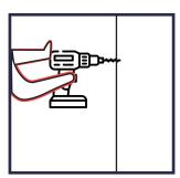
Once you have your marks. Drill into the tile firmly with two hands. The holes should be just smaller than the screws
