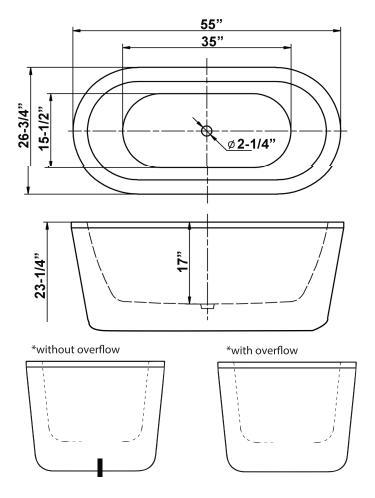
\*rough in center line 1" inch off outside of tub
