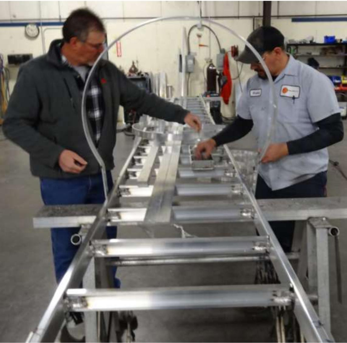
3. Place bottom ring upright on the first set of holes from the bottom of the ladder (typically 7'-6" from bottom).
