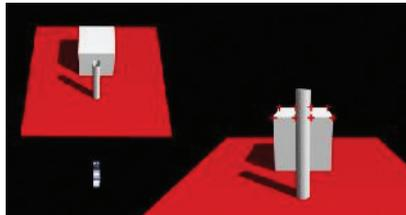
In following diagram, the camera has moved up and right. This movement would be accurately calculated if just the features at the corners of the cube were used. However, the T-junctions have moved very little since the first frame and their contribution would result in an inaccurate solve. In reality there would be far more features tracked in this scene; the T-junctions would be discarded because their motion is inconsistent with the rest of the tracks.
