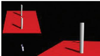
The following diagram shows the effect of panning the camera left and trucking it to the right. The camera's center is now at a different position in 3D space and it can see the second cylinder.
