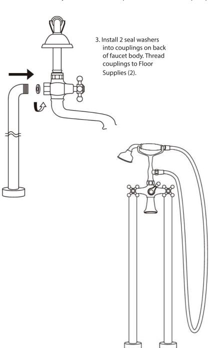
4.Connect the Handshower Hose (6) to both the Handshower and Faucet Body (2). Connect to water supply beneath floor and turn faucet on to test for leaks. Test all 3 handles to ensure water connections for hot and cold are correct and diverter for handshower works properly.
