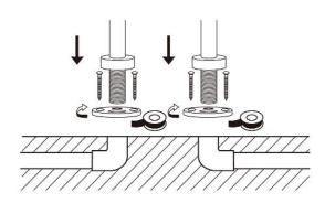
2. Wrap threaded ends of Bath Supplies (2) with teflon tape and thread through Cover Plates (4). Secure Cover Plates (4) to floor with Screws (5) provided. Thread enough through floor to ensure water connections can be done while testing height to ensure proper placement of tub filler over tub rim. Slide Floor Escutcheons (3) down to conceal Cover Plates.
