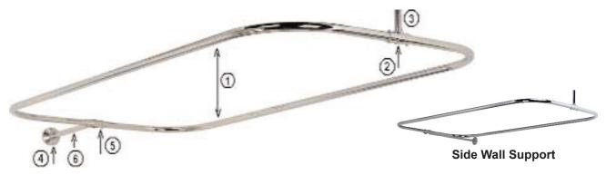
Connect both halves of the curtain frame (1) using the ceiling tees and wall tees as shown above. In order to insure a solid fit, the tees fit snugly over the frame tube. Install 4 set screws in each tee.
