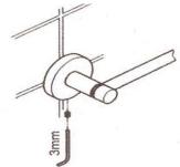
5. Secure accessory to bracket using set screws and allen wrench provided.
