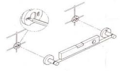
**1.** Hold accessory to desired location on wall. Mark wall for mounting brackets.
