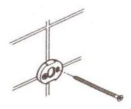
Screw mounting brackets securely to wall.
