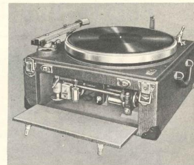
Overhead mechanism is carried inside case.
