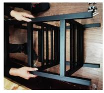
Take the remaining set of legs and carefully insert the brackets into the shelves and bar. Up to this point, no hardware has been used.
