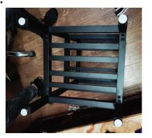
Flip the stabd so that the legs are in the air and the straight bar is on the ground. Screw the leveling feet into the legs of the stand. These can be adjusted to ensure a level sink.
