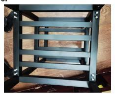
Screw the short silver screws into the shelves on the underside. There are eight screws per shelf and four for the bar at the top.
