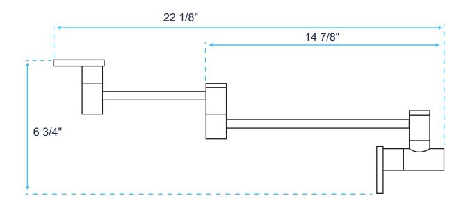
2 3/8" Length (Measured at Base Plate) 6 3/4" Height 22 1/8" Spout Reach
