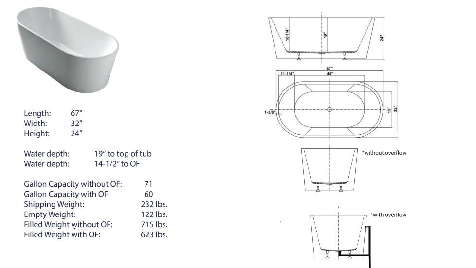
\*rough in center line 1" inch off outside of tub
